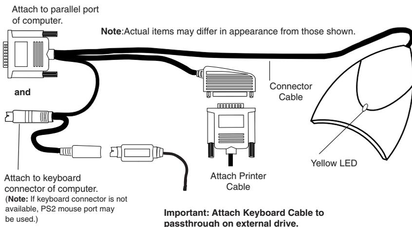
Follow the computer shutdown procedure, and turn off your printer and any parallel port device(s). Remove any printer cable (or other device cable) attached to your parallel port. Attach the external drive cables to the parallel port and keyboard connector of your computer. Make sure to attach the keyboard cable to the external drive keyboard cable passthrough.
